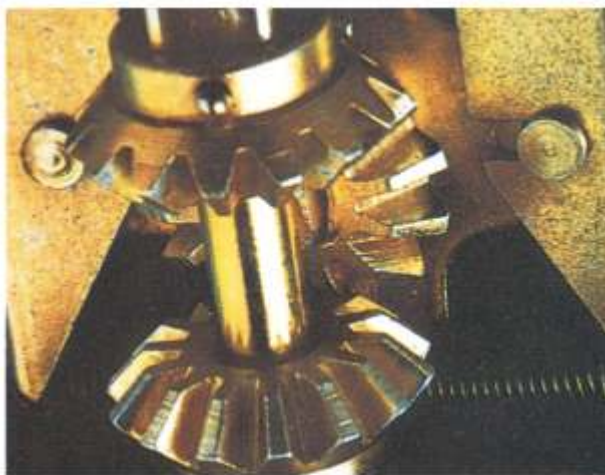
The operating mechanism in ratings of 200A to 1000A uses a Bevel gear system.
